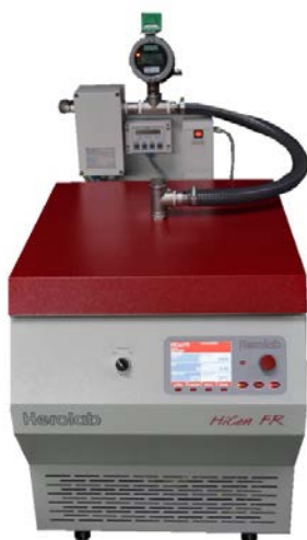
Photo: Floor centrifuge HiCen FR with Inert Gas Purging system
